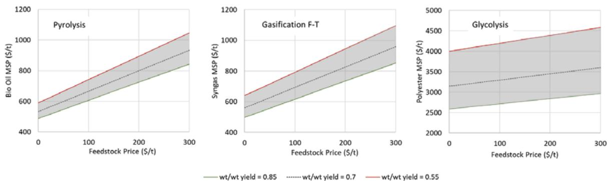
Figure 8: Impact of assumed product yield on the MSP for: pyrolysis, gasification and glycolysis.
