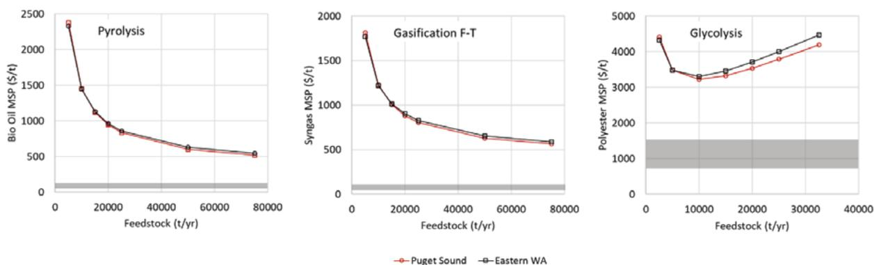
**Figure 6: Impact of facility scale on MSP for pyrolysis, gasification and glycolysis recycling operations.**
