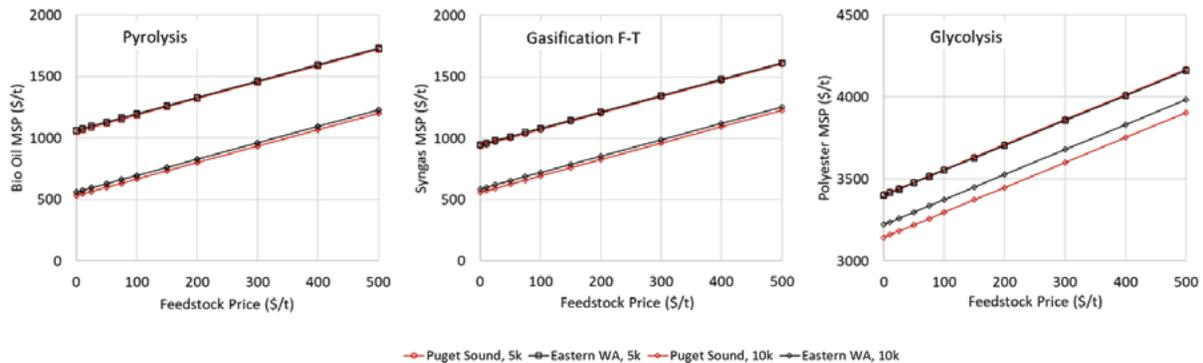
Figure 7: Impact of feedstock price on MSP for baseline scale pyrolysis, gasification and glycolysis facilities at two locations and facility scales.
