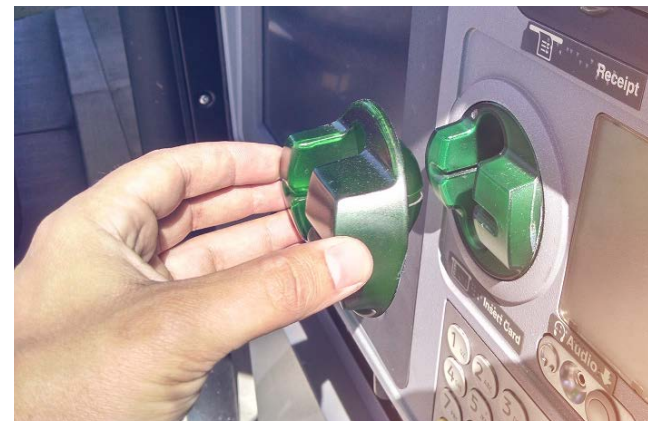
A skimmer being installed on an ATM
